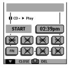
7. Tap the clock button on the right and set the start time using the Left/Right buttons.
